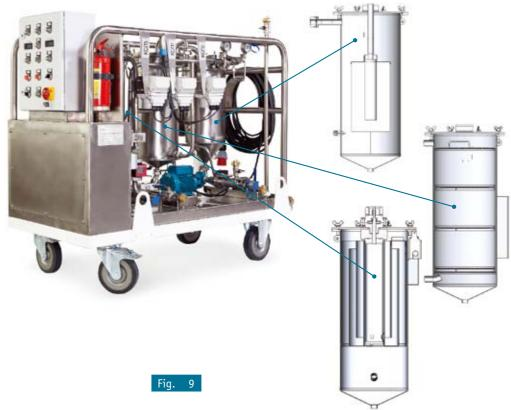
The oil cleaner can operate in two different modes depending on the presence or absence of water in the oil to be cleaned (water content is detected automatically).
