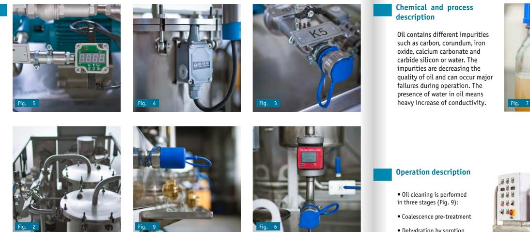
All components in contact with non-conductive fluid are made of materials resistant to aggressive substances (stainless steel, oil and petrol resistant rubber, etc.) (Fig. 2).
