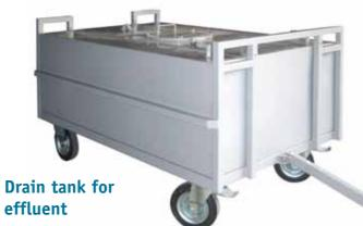
A mobile unit for recovery, storage and transportation of drainage liquid after compressor cleaning to the waste recycling facility
